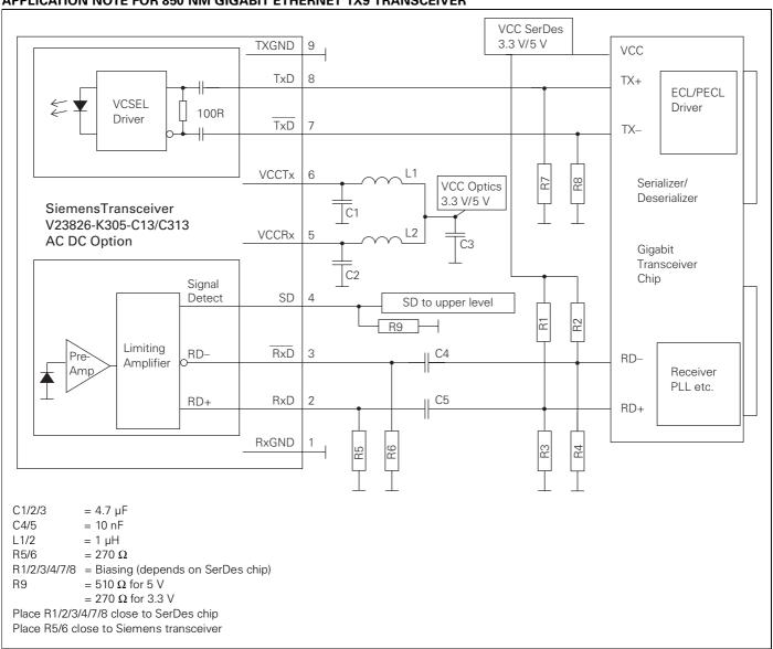
Values of R1/2/3/4 may vary as long as proper 50  $\Omega$  termination to  $V_{EE}$  or 100  $\Omega$  differential is provided. The power supply filtering is required for good EMI performance. Use short tracks from the inductor L1/L2 to the module  $V_{CC}RX/V_{CC}TX$ .
