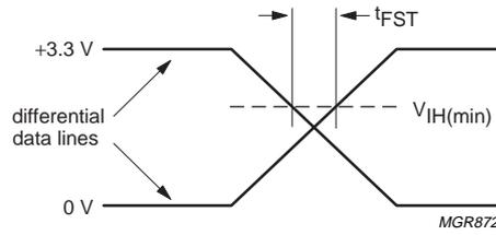
Fig 18. Receiver SE0 width tolerance.
