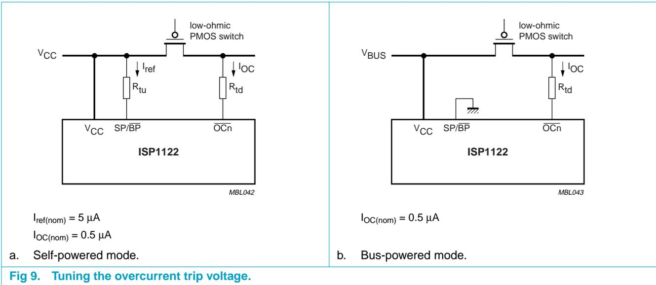
Fig 9. Tuning the overcurrent trip voltage.
