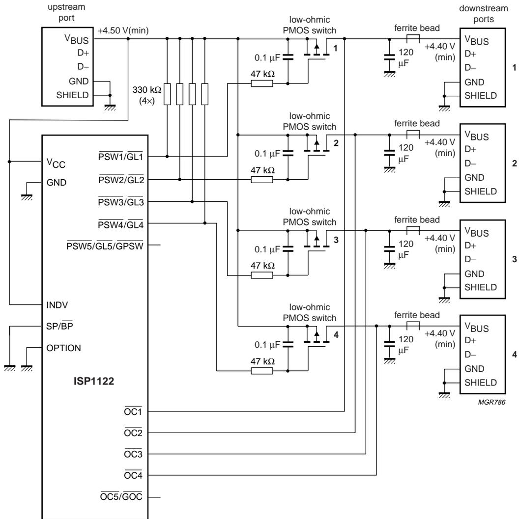
Power switches 1 to 4 are low-ohmic PMOS devices as specified in [Section 12.2](#).
