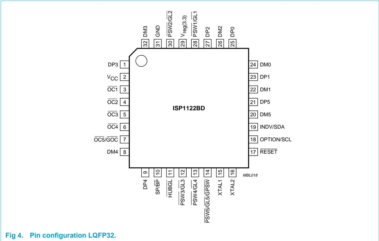
Fig 4. Pin configuration LQFP32.
