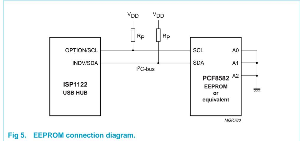
Fig 5. EEPROM connection diagram.
