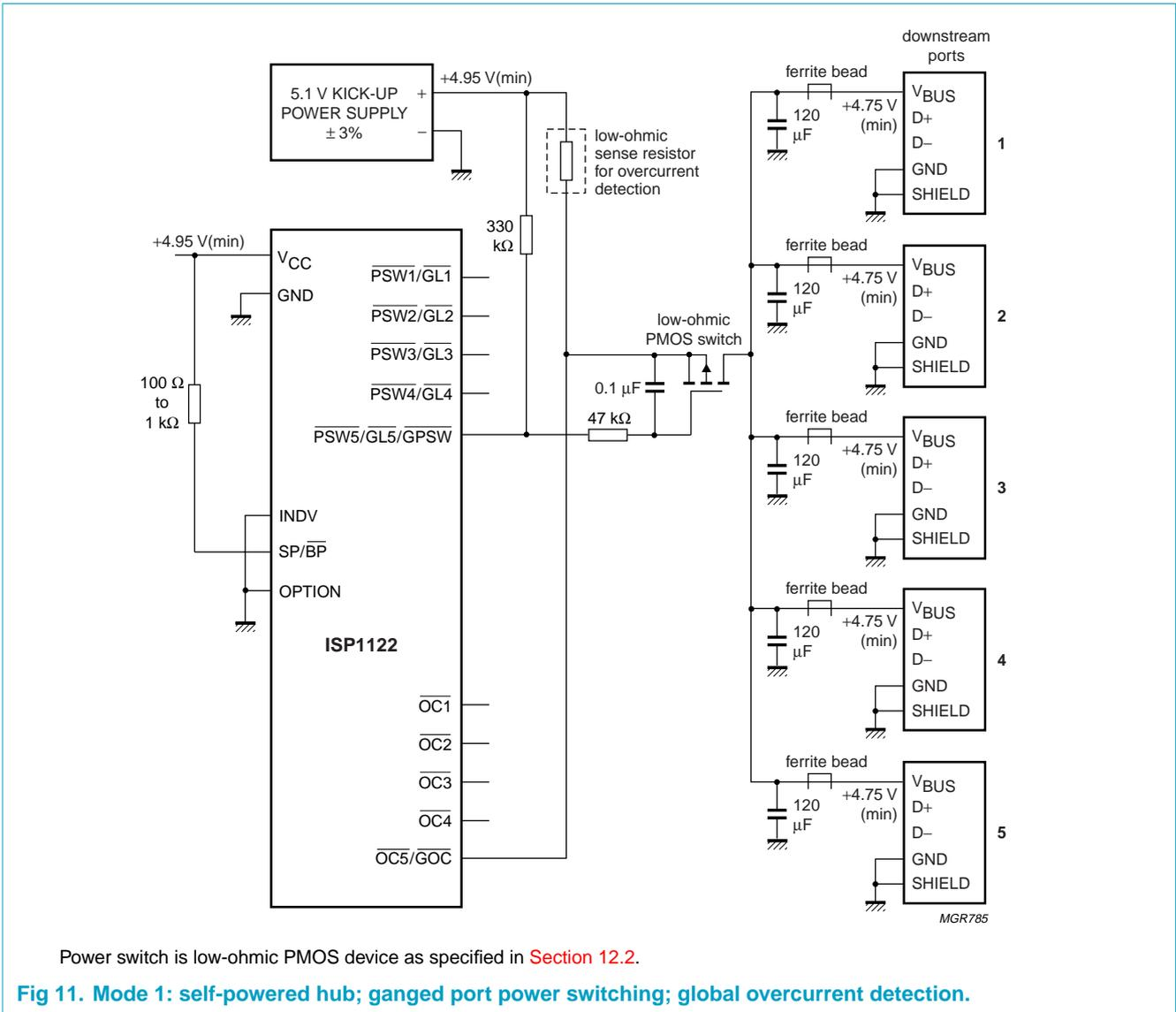
Power switch is low-ohmic PMOS device as specified in Section 12.2.
