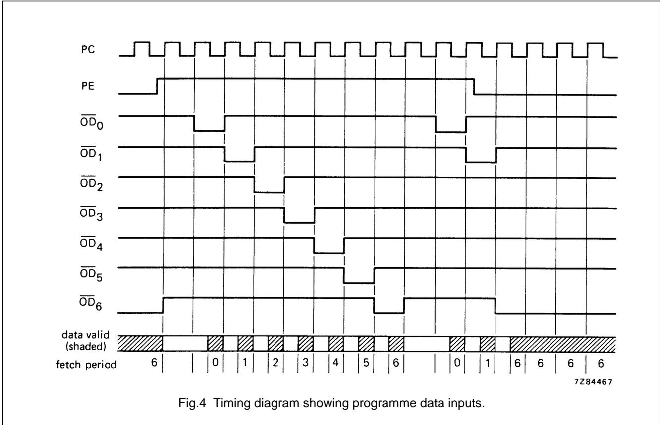
Fig.4 Timing diagram showing programme data inputs.
