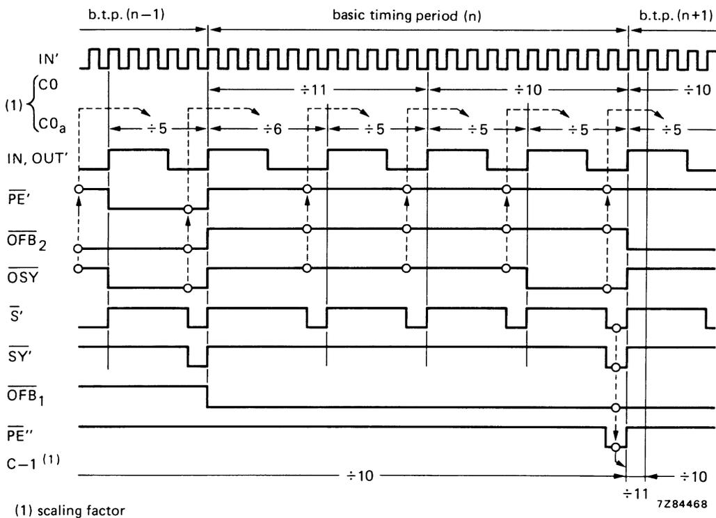
Fig.6 Timing diagram showing signals occurring in Fig.5.
