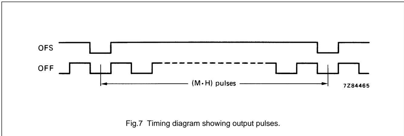
Fig.7 Timing diagram showing output pulses.
