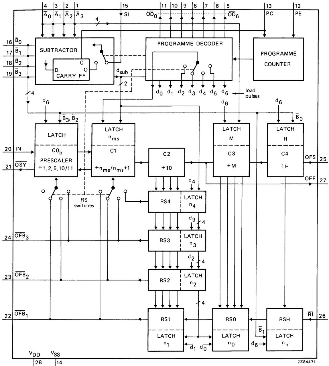
Fig.2 Block diagram.
