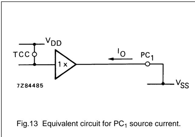
Fig.13 Equivalent circuit for PC<sub>1</sub> source current.
