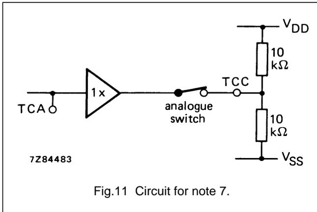
Fig.11 Circuit for note 7.
