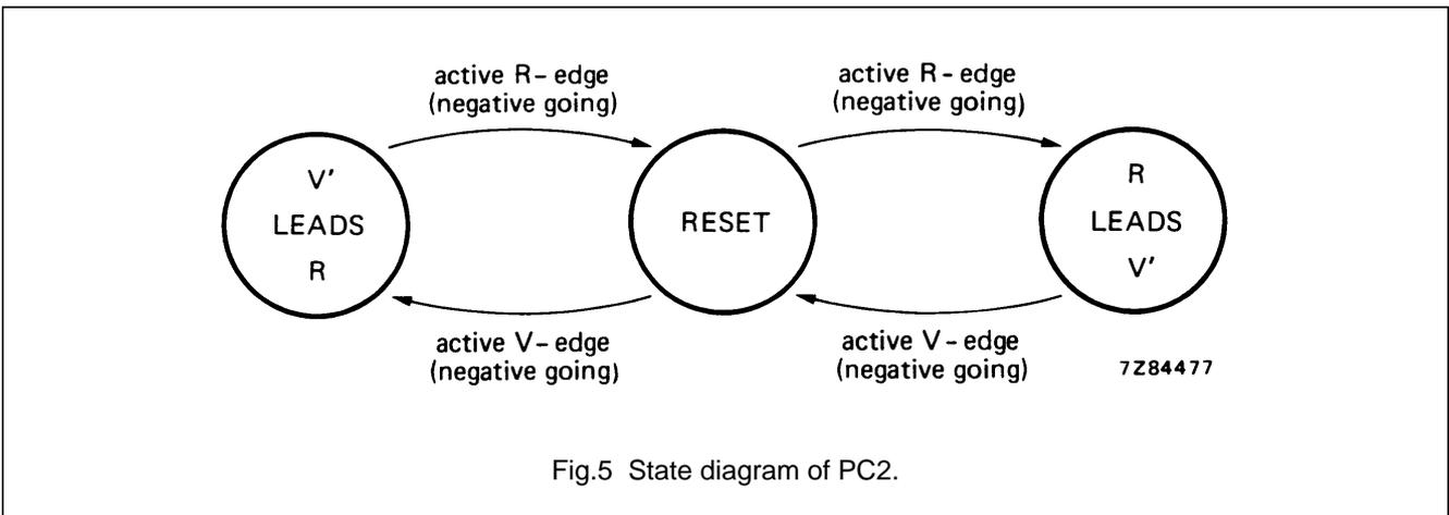
Output PC<sub>2</sub> produces positive or negative-going pulses with variable width; they depend on the phase relationship of R and V'. The average output voltage is a linear function of the phase difference. Output PC<sub>2</sub> remains in the high impedance OFF-state in the region in which PC1 operates. The resultant phase characteristic is shown in Fig.6.
