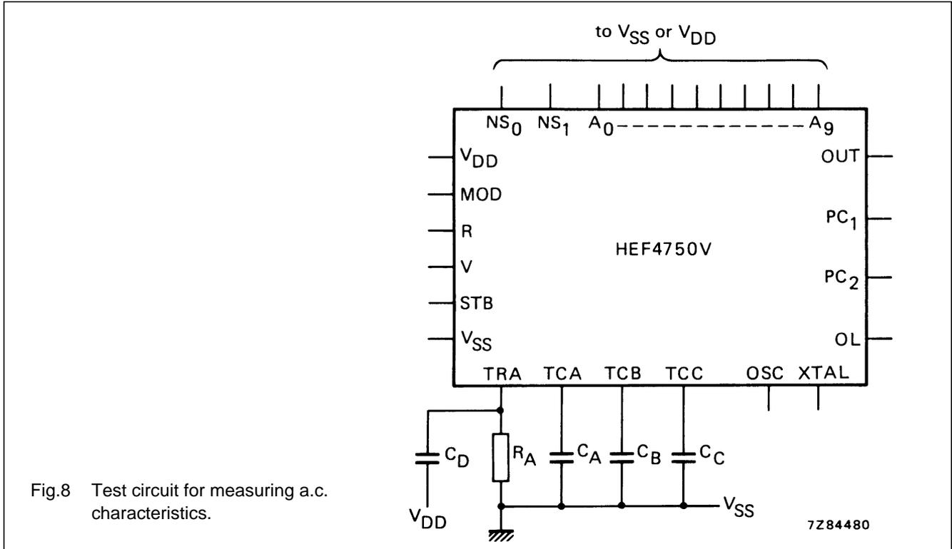
Fig.8 Test circuit for measuring a.c. characteristics.
