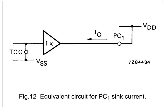
Fig.12 Equivalent circuit for PC1 sink current.
