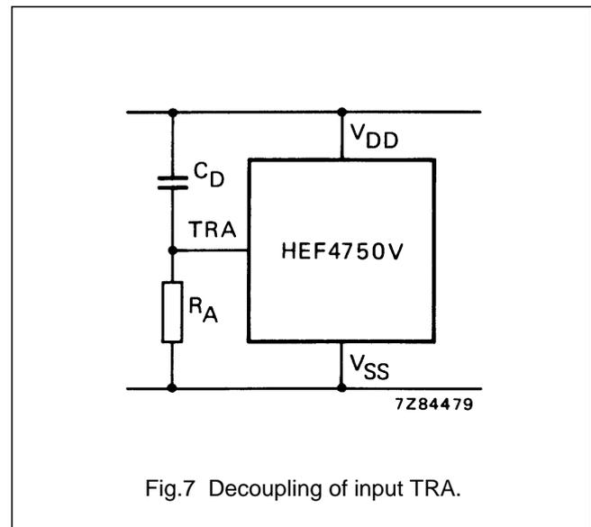
Fig.7 Decoupling of input TRA.
