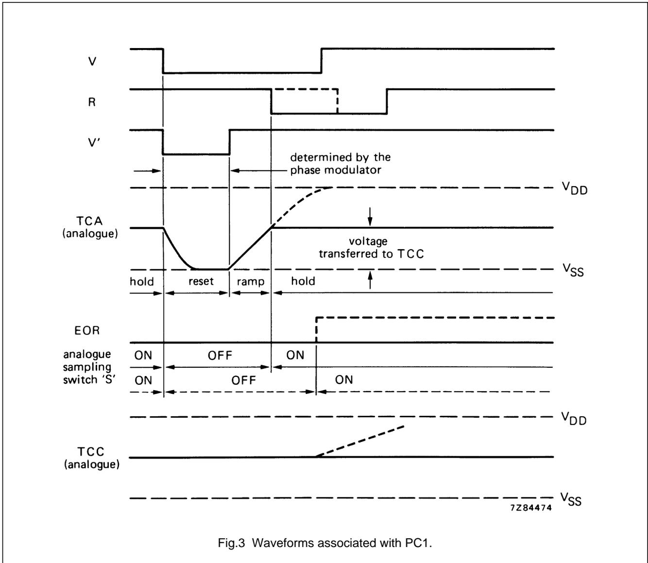
Fig.3 Waveforms associated with PC1.
