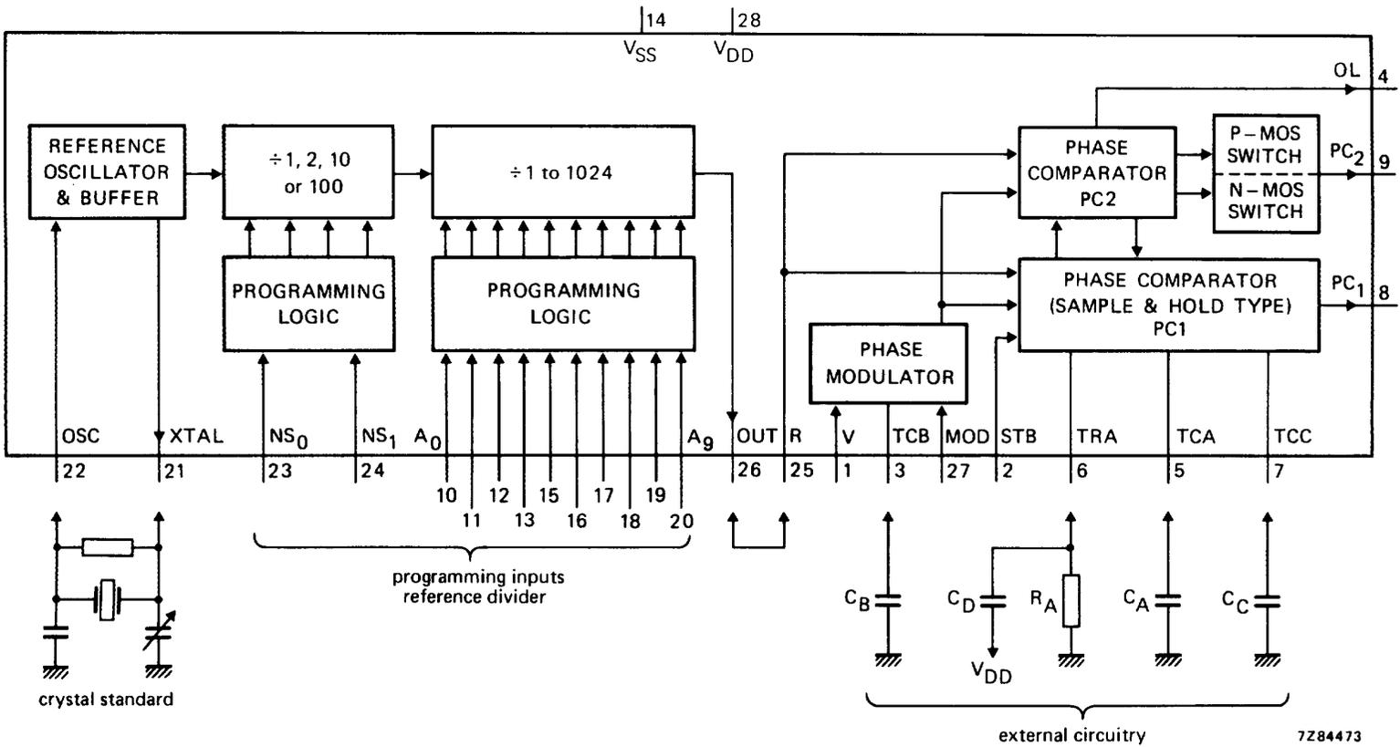
N.B. PC<sub>1</sub> = analogue output; PC<sub>2</sub> = 3-state output.
