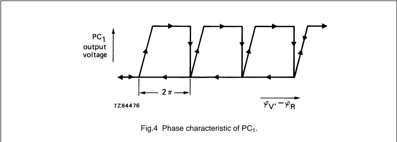
PC1 is designed to have a high gain, typically 3200 V/cycle (at 12,5 kHz). This enables a low noise performance.
