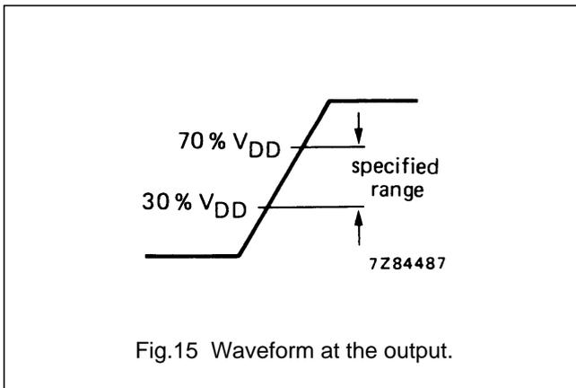
Fig.15 Waveform at the output.
