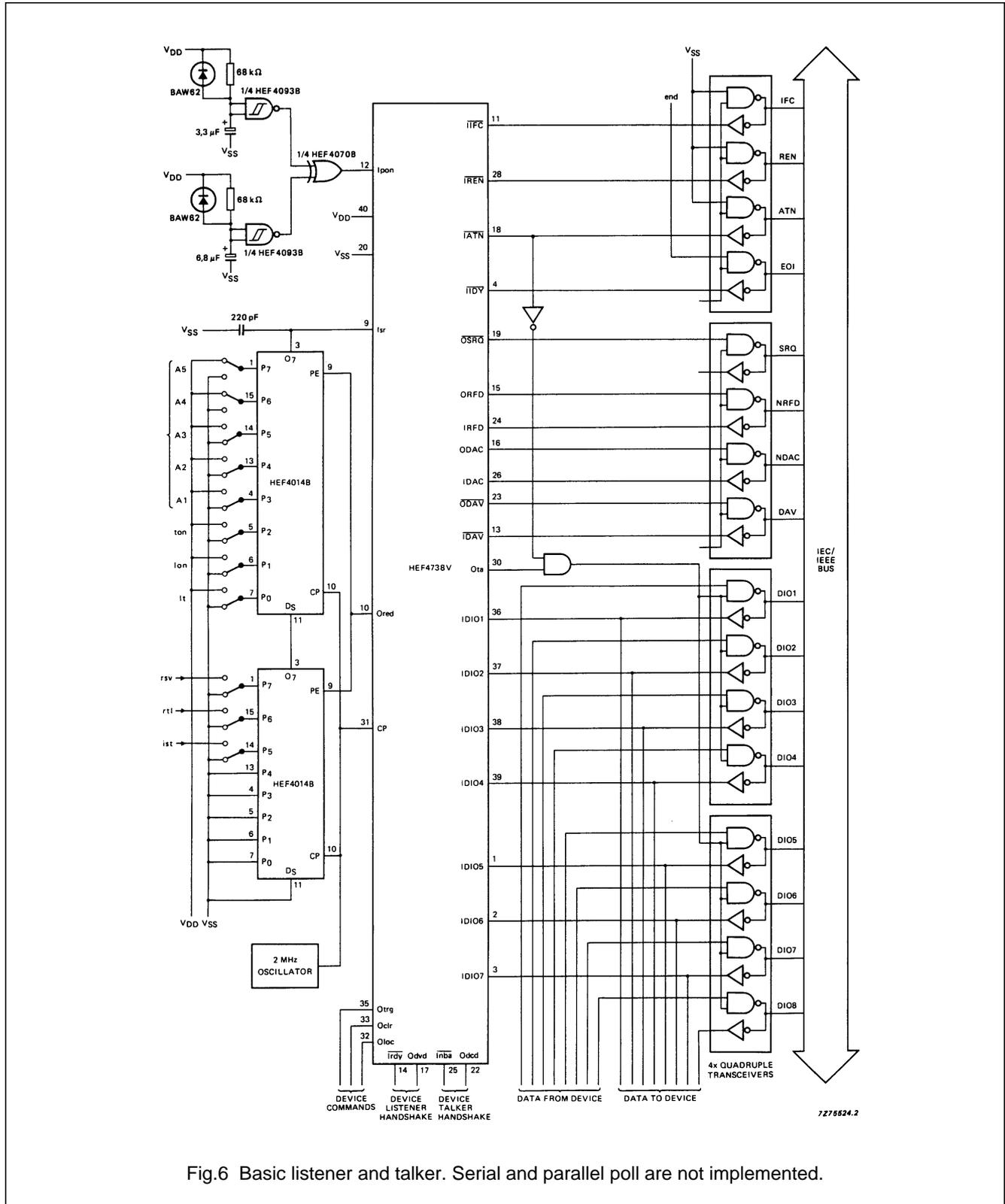
Fig.6 Basic listener and talker. Serial and parallel poll are not implemented.
