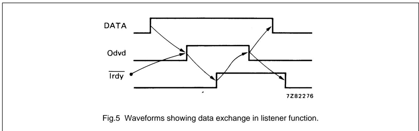
Fig.5 Waveforms showing data exchange in listener function.
