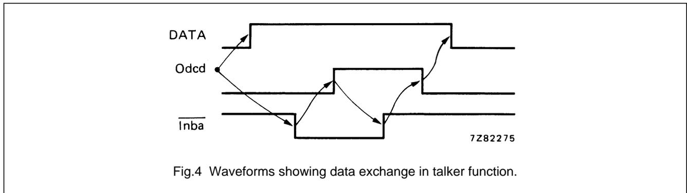
Fig.4 Waveforms showing data exchange in talker function.
