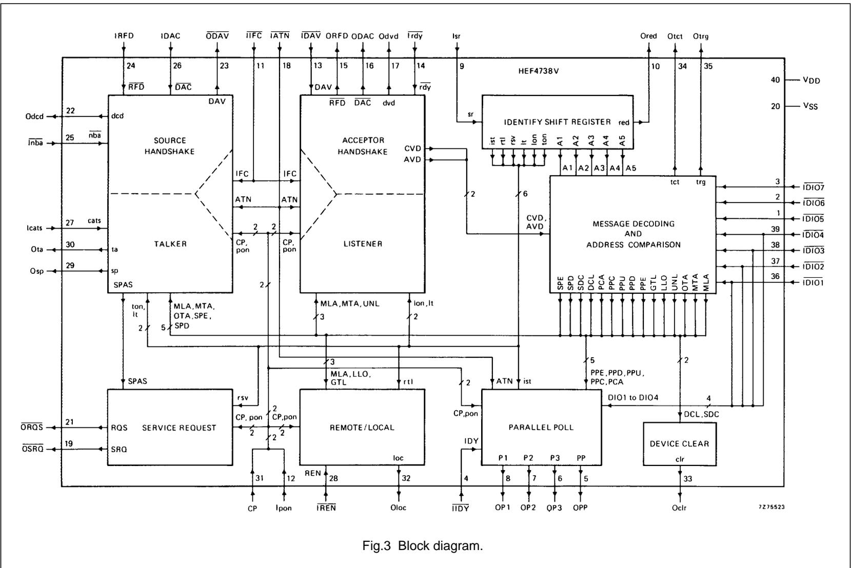
Fig.3 Block diagram.
