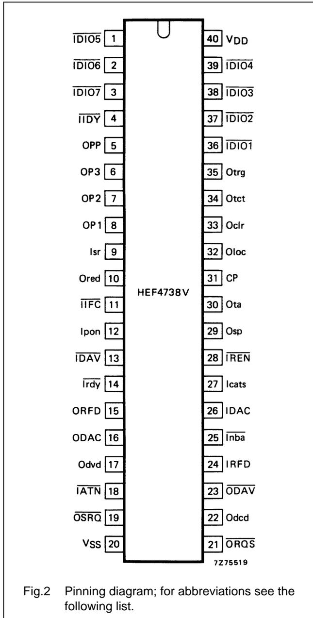
Fig.2 Pinning diagram; for abbreviations see the following list.
