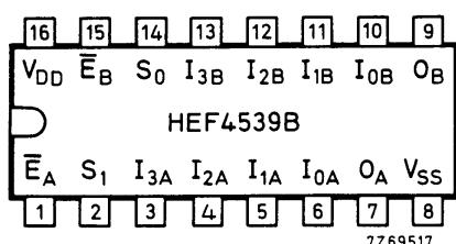
Fig.2 Pinning diagram.
