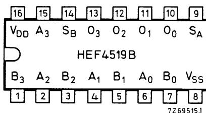
Fig.2 Pinning diagram.
