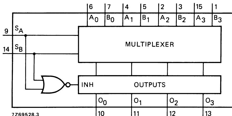
Fig.1 Functional diagram.
