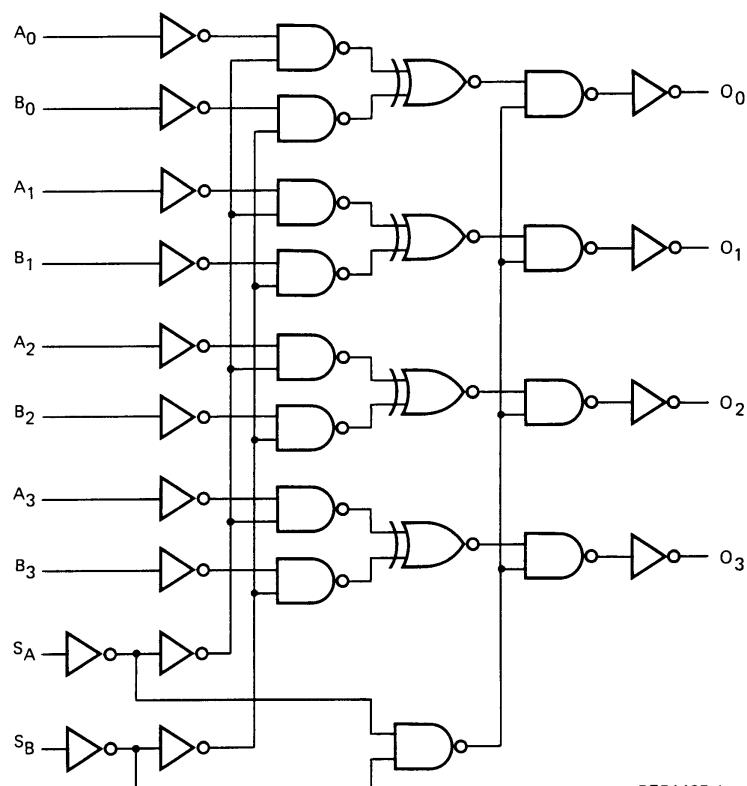
Fig.3 Logic diagram.
