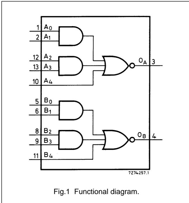
Fig.1 Functional diagram.
