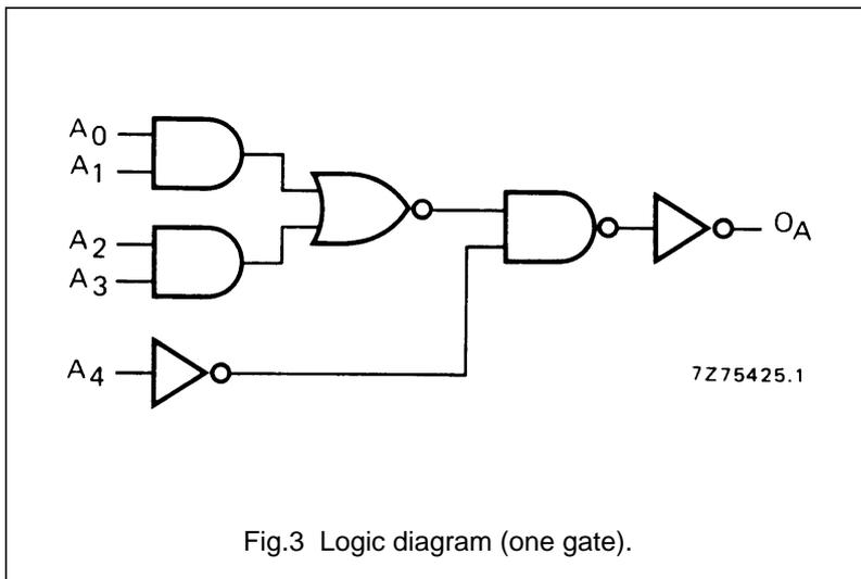
Fig.3 Logic diagram (one gate).
