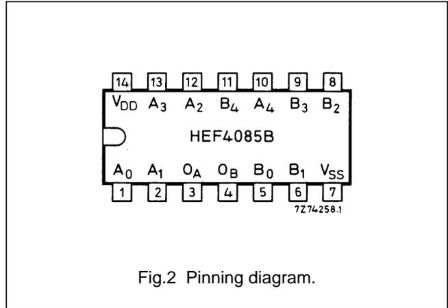
Fig.2 Pinning diagram.
