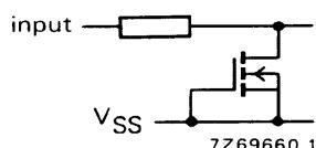
Fig.4 Input protection circuit that allows input voltages in excess of  $V_{DD}$ .**FAMILY DATA,  $I_{DD}$  LIMITS category BUFFERS**
