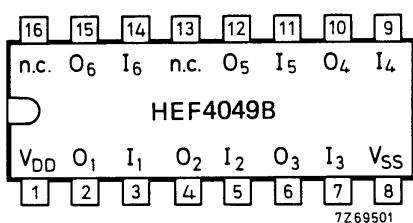
Fig.2 Pinning diagram.
