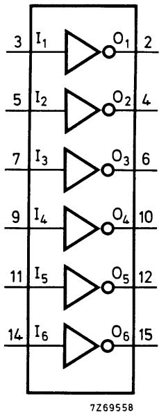
Fig.1 Functional diagram.
