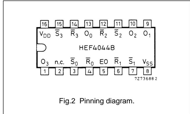
Fig.2 Pinning diagram.
