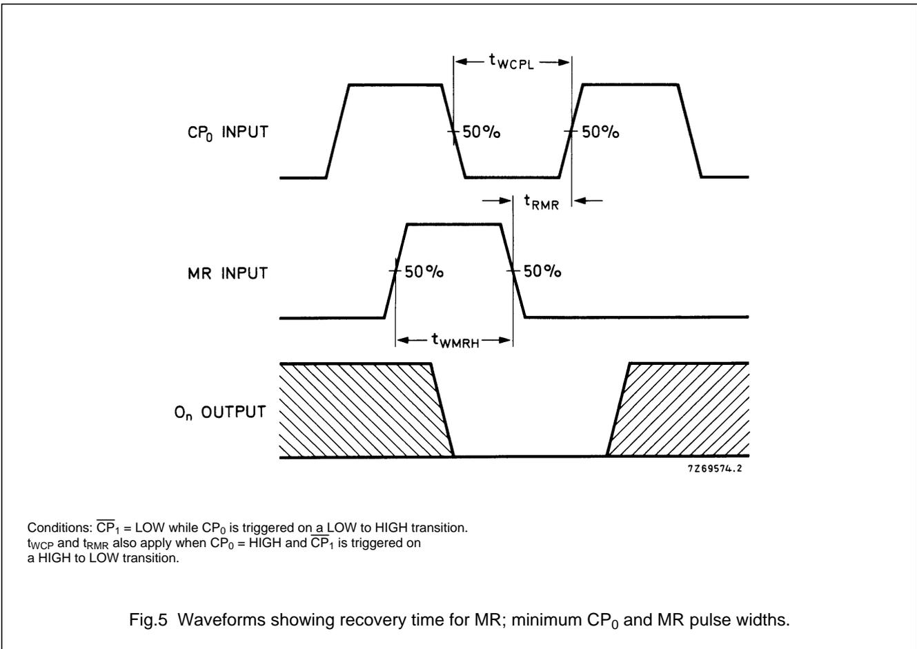
Conditions:  $\overline{CP}_1 = \text{LOW}$  while CP<sub>0</sub> is triggered on a LOW to HIGH transition.
