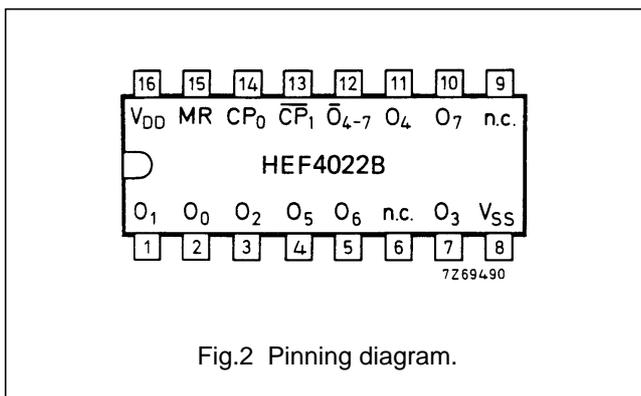
Fig.2 Pinning diagram.
