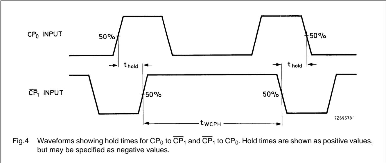
Fig.4 Waveforms showing hold times for CP<sub>0</sub> to  $\overline{CP}_1$  and  $\overline{CP}_1$  to CP<sub>0</sub>. Hold times are shown as positive values, but may be specified as negative values.
