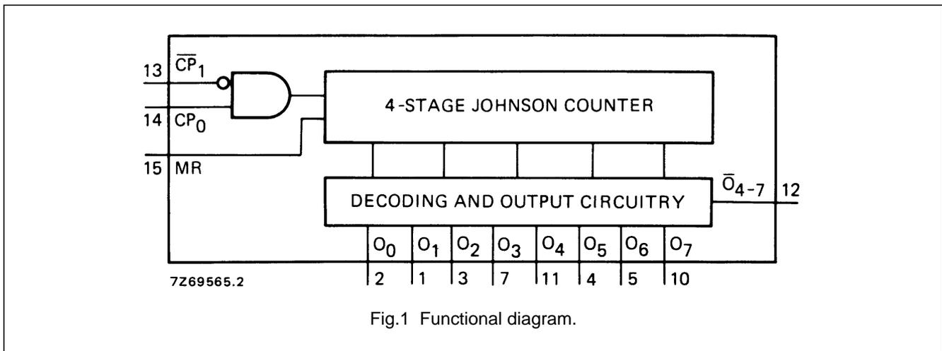
Fig.1 Functional diagram.
