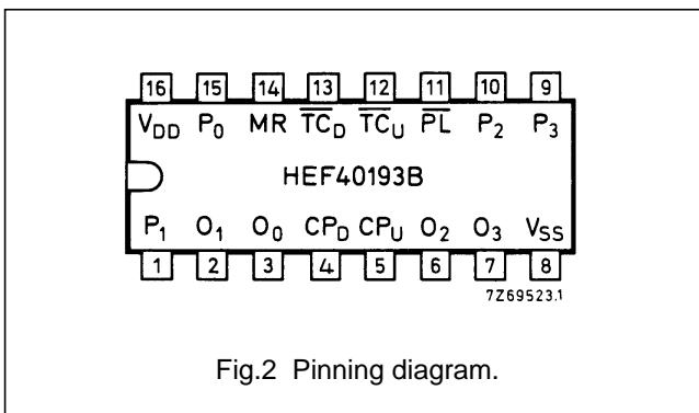
Fig.2 Pinning diagram.
