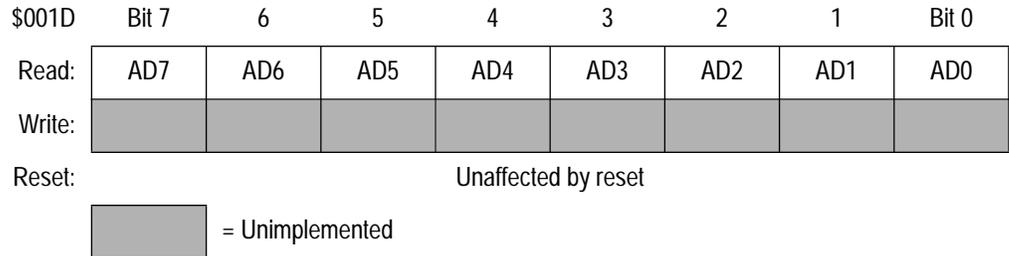
**Figure 9-2. A/D Conversion Value Data Register (ADC)**
