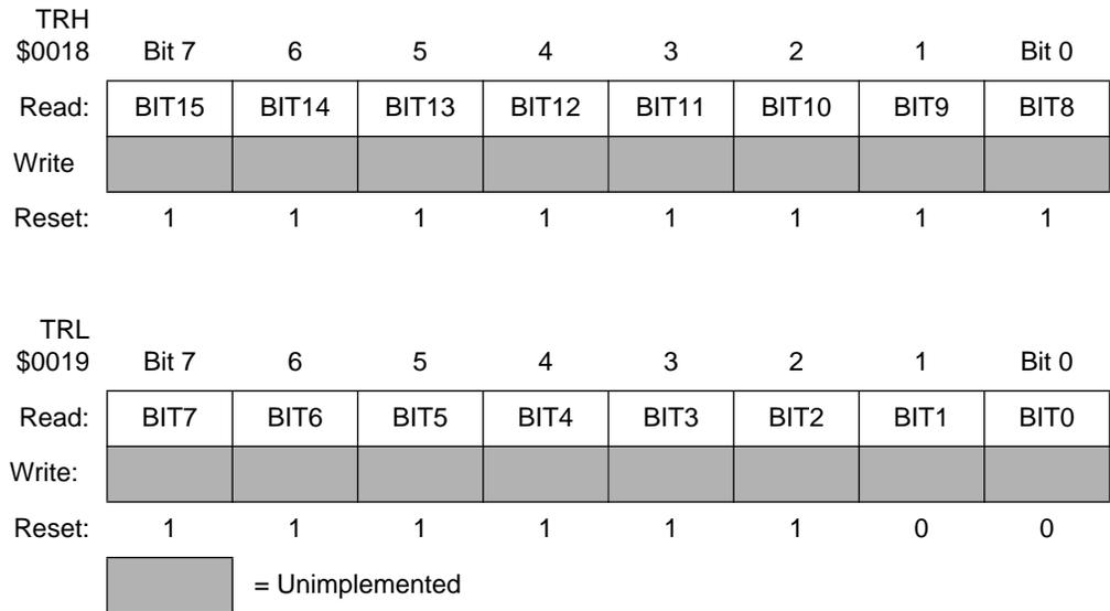
**Figure 8-4. Timer Registers (TRH and TRL)**
