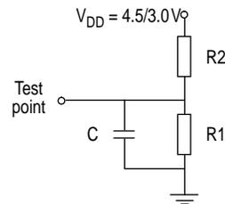
**Figure 11-1** Equivalent test load
