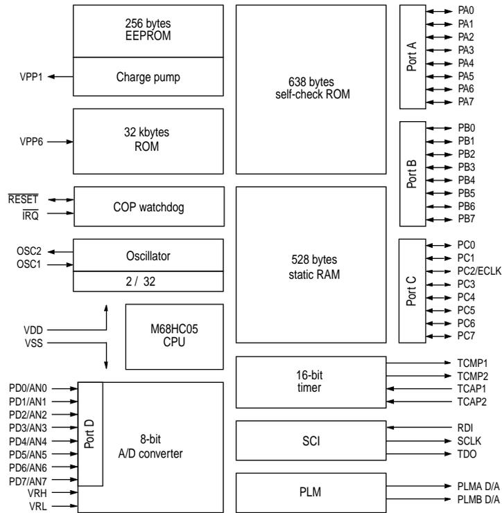
Figure F-1 MC68HC05B32 block diagram
