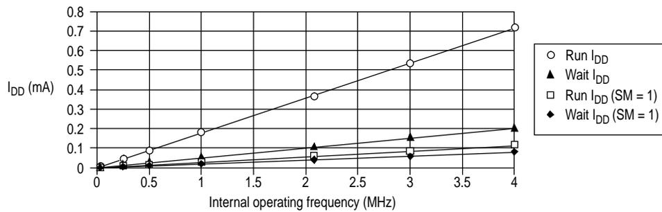
**Figure 11-7** I<sub>DD</sub> vs mode vs internal operating frequency, V<sub>DD</sub> = 5.5V
