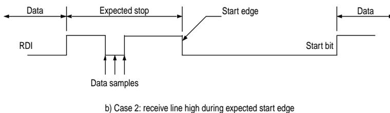
**Figure 6-6** Artificial start following a framing error
