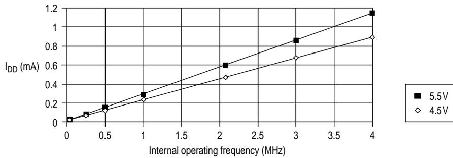
Figure 11-3 Run I<sub>DD</sub> (SM = 1) vs internal operating frequency (4.5V, 5.5V)
