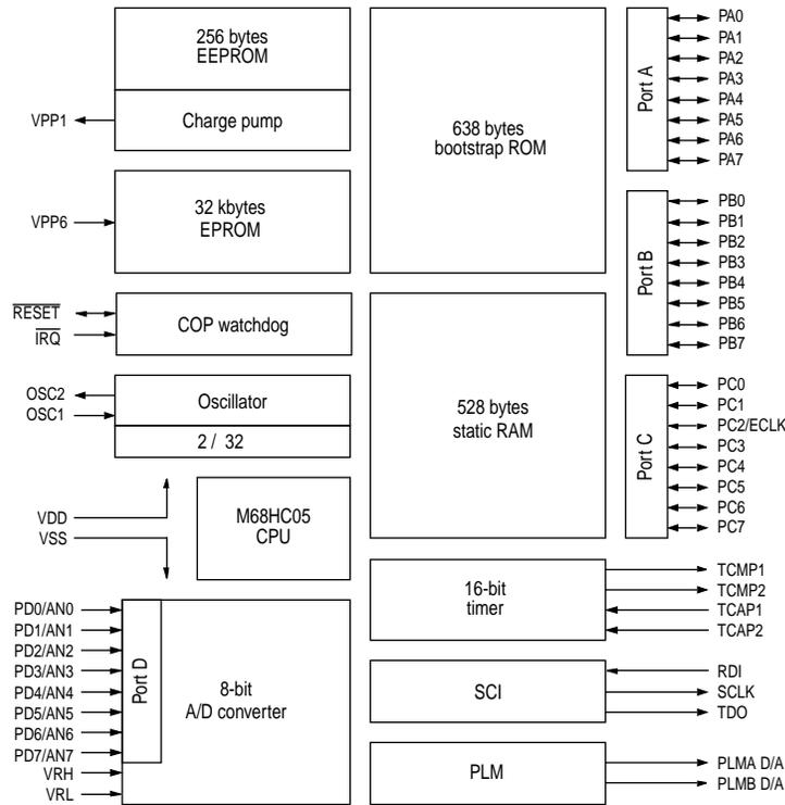
**Figure G-1** MC68HC705B32 block diagram
