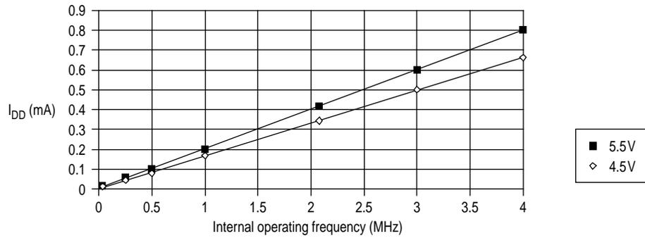
**Figure 11-5** Wait I<sub>DD</sub> (SM = 1) vs internal operating frequency (4.5V, 5.5V)
