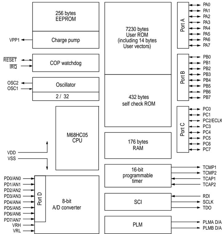
Figure B-1 MC68HC05B8 block diagram
