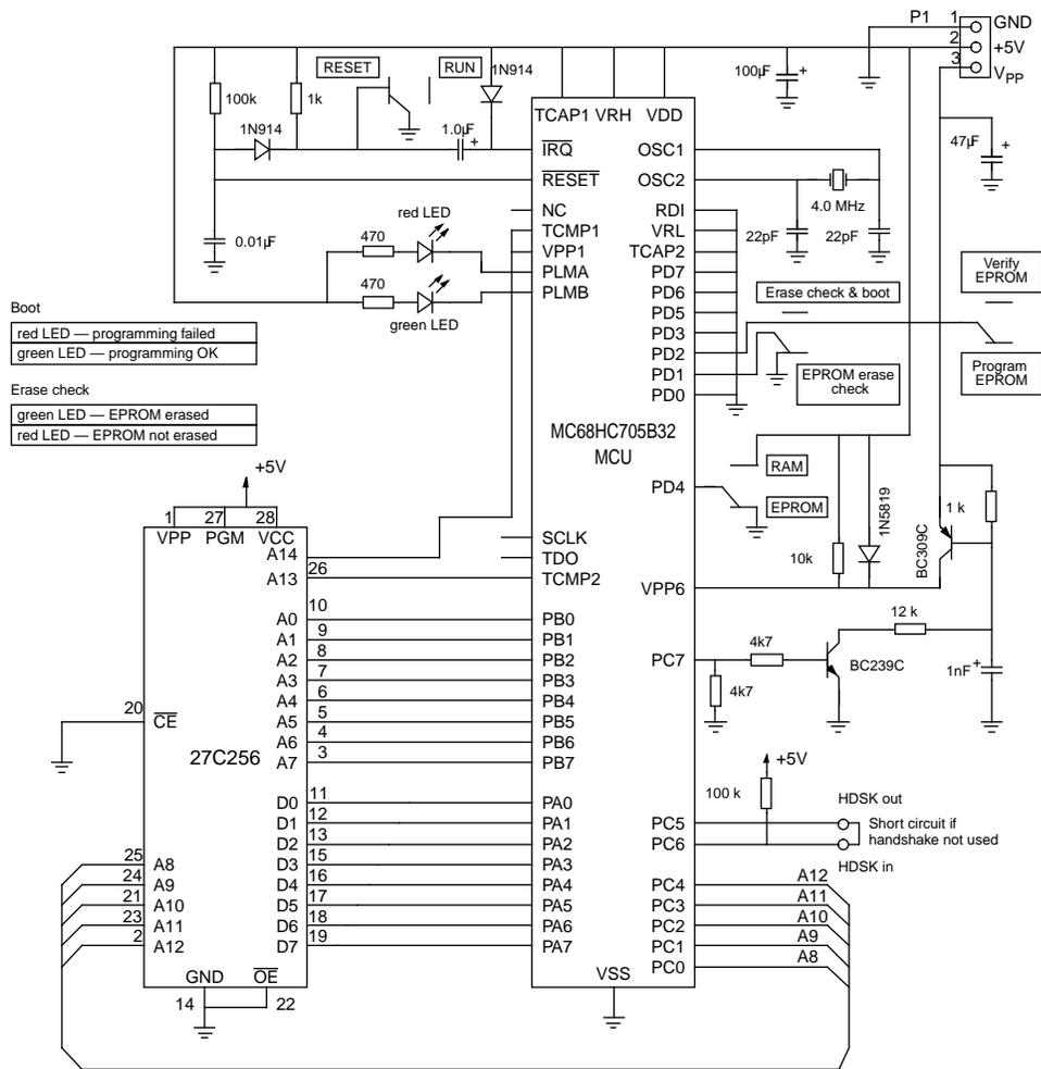
Figure G-7 EPROM parallel bootstrap schematic diagram
