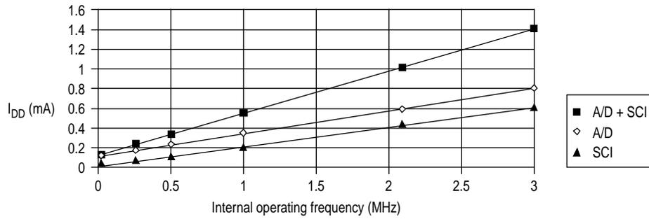
**Figure 11-6** Increase in I<sub>DD</sub> vs frequency for A/D, SCI systems active, V<sub>DD</sub> = 5.5V
