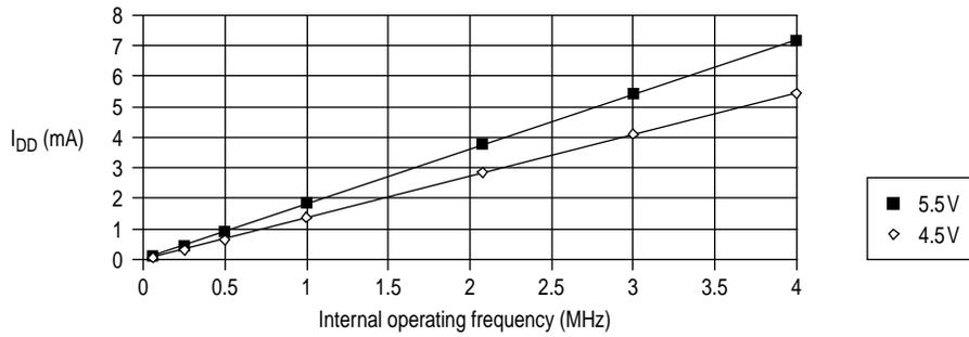
Figure 11-2 Run I<sub>DD</sub> vs internal operating frequency (4.5V, 5.5V)
