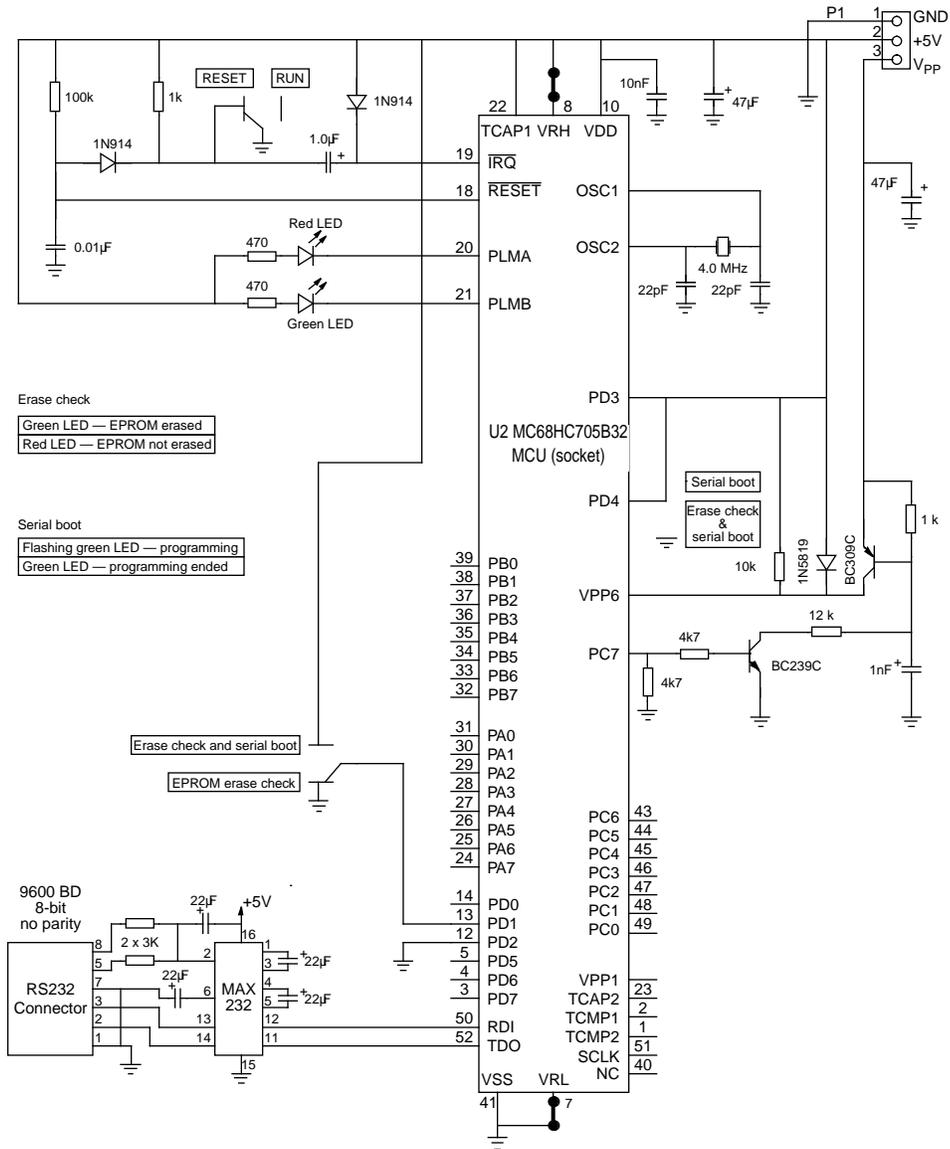
Figure G-8 RAM load and execute schematic diagram
