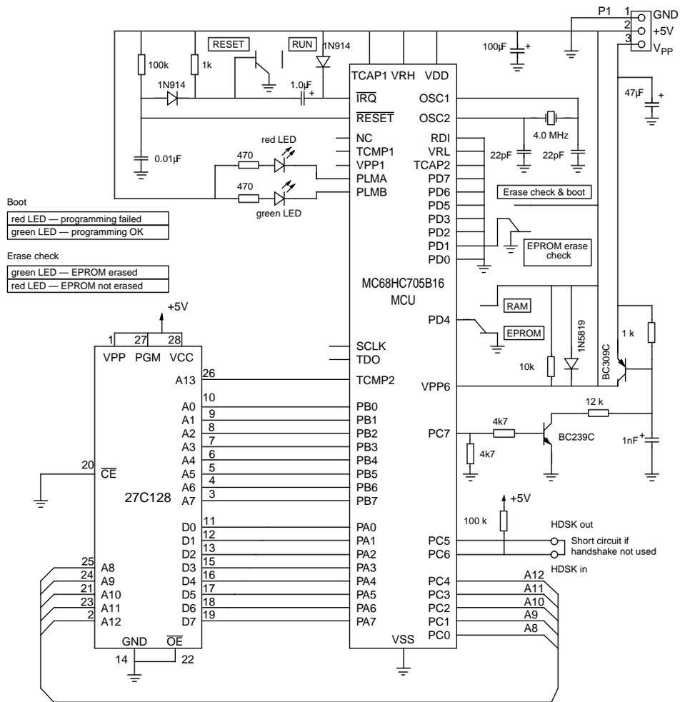
Figure E-7 EPROM Parallel bootstrap schematic diagram
