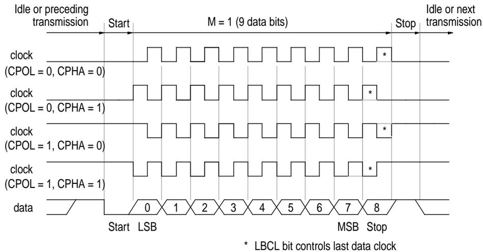
**Figure 6-10** SCI data clock timing diagram (M=1)
