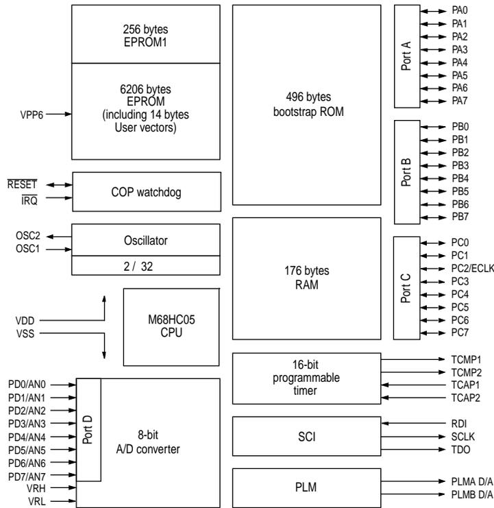
Figure C-1 MC68HC705B5 block diagram
