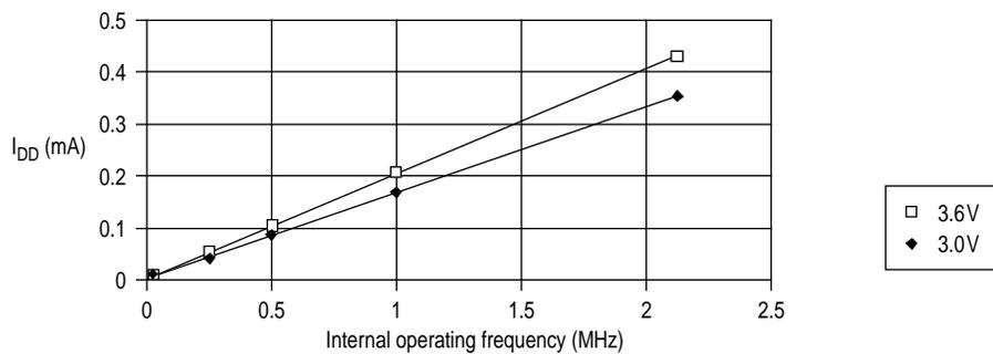
**Figure 11-11** Wait I<sub>DD</sub> (SM = 1) vs internal operating frequency (3V, 3.6V)
