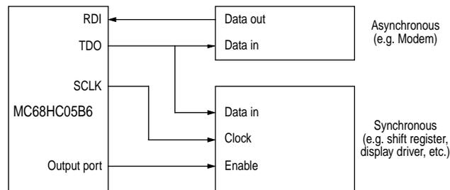
Figure 6-8 SCI example of synchronous and asynchronous transmission
