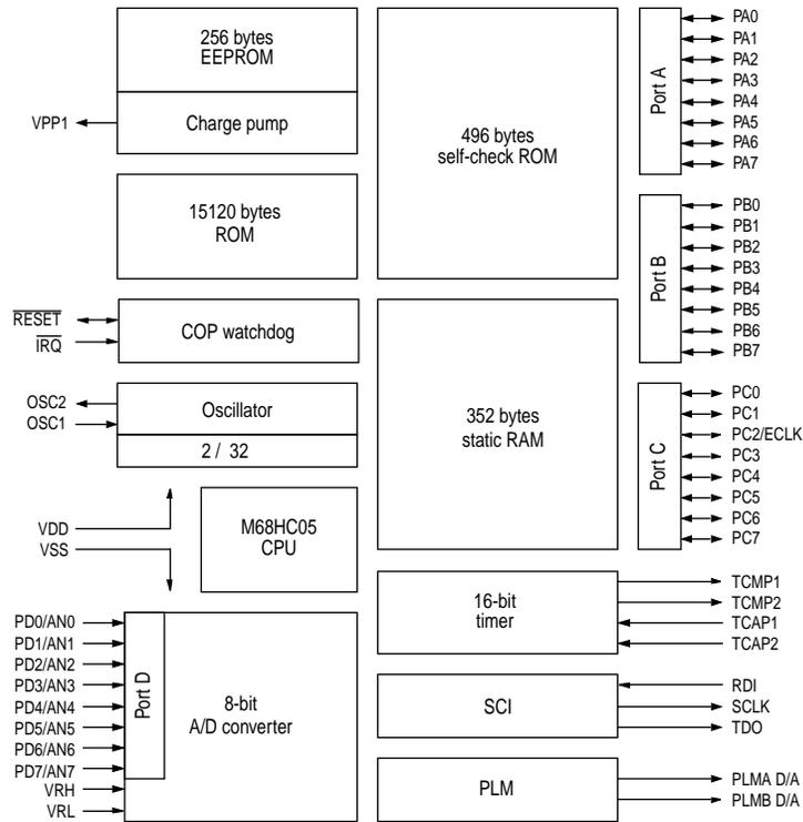
Figure D-1 MC68HC05B16 block diagram
