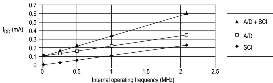
**Figure 11-12** Increase in I<sub>DD</sub> vs frequency for A/D, SCI systems active, V<sub>DD</sub> = 3.6V
