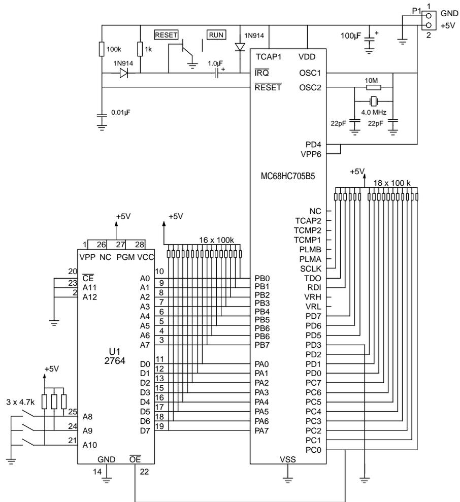
Figure C-8 RAM parallel bootstrap schematic diagram
