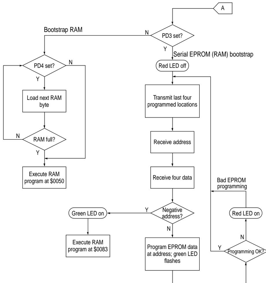
Figure C-4 Modes of operation flow chart (2 of 2)
