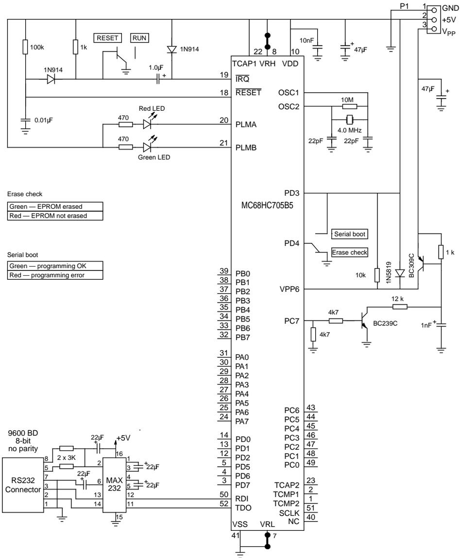
Figure C-7 EPROM (RAM) serial bootstrap schematic diagram
