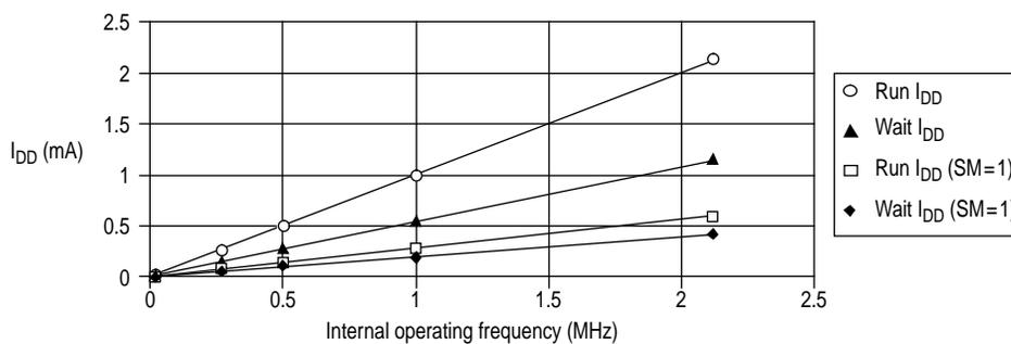
**Figure 11-13** I<sub>DD</sub> vs mode vs internal operating frequency, V<sub>DD</sub> = 3.6V
