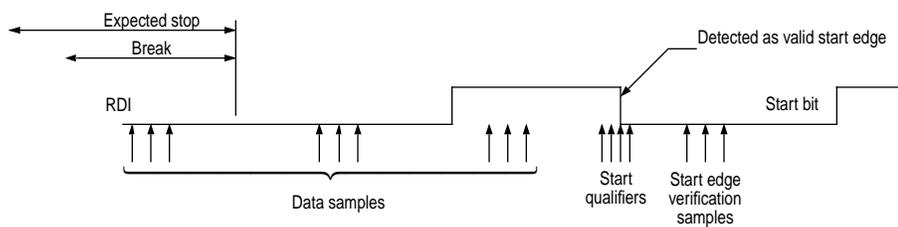
**Figure 6-7** SCI start bit following a break
