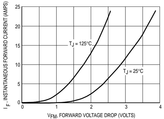
**Figure 10. Maximum Forward Drop versus Instantaneous Forward Current**
