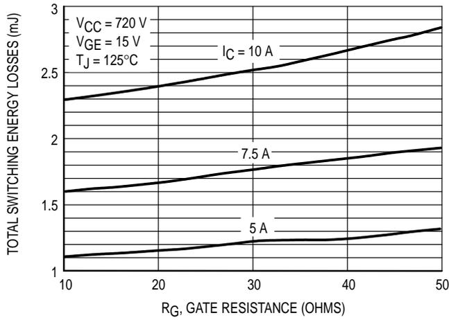
**Figure 7. Total Switching Losses versus Gate Resistance**
