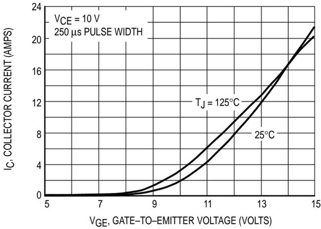
Figure 3. Transfer Characteristics
