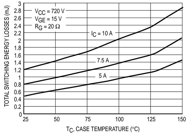
**Figure 8. Total Switching Losses versus Case Temperature**
