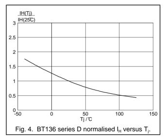
$I_{H}$  increases for the larger E series triacs. The most sensitive D series triacs, however, are designed to maintain a consistent, low  $I_{H}$  of 10mA @ 25°C even for the higher 8A current rating.
