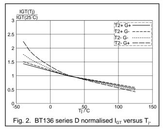
Since the control IC operates on a single rail supply (usually +5V), its outputs are unipolar. It can be referenced to the mains circuit in order to source current (positive gate drive) or to sink current (negative gate drive). Since 4th quadrant triggering should be avoided, optimum performance will be obtained with negative gate current - i.e operation in the 2nd (T2+, G-) and 3rd (T2-, G-) quadrants (see Fig. 1).
