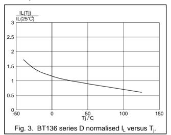
How quickly the load current reaches the triac's  $I_{L}$  will depend on the peak load current and mains frequency. Taken to the extreme case, if the load current is so low that its peak value is equivalent to  $I_{L}$ , it will take one quarter cycle, or 5ms for 50Hz mains, before the triac is latched and the gate pulse can cease.
