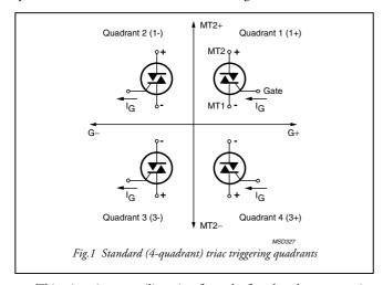
This triggering versatility arises from the fact that the gate consists of some elements that conduct temporarily during the turn-on phase. In particular, one of the triggering modes, 3+ (or quadrant 4), relies
