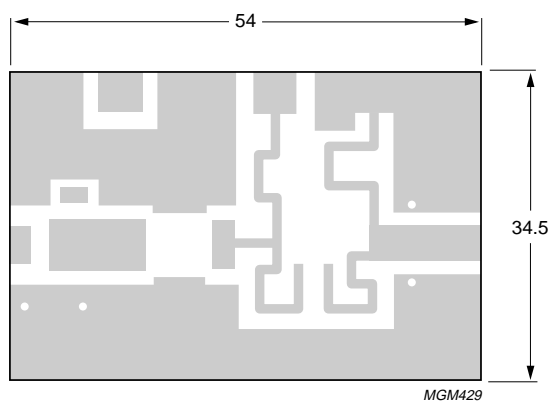
Fig.13 Printed-circuit board BLW32.
