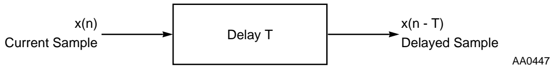
Figure C-3 Single Delay Line
