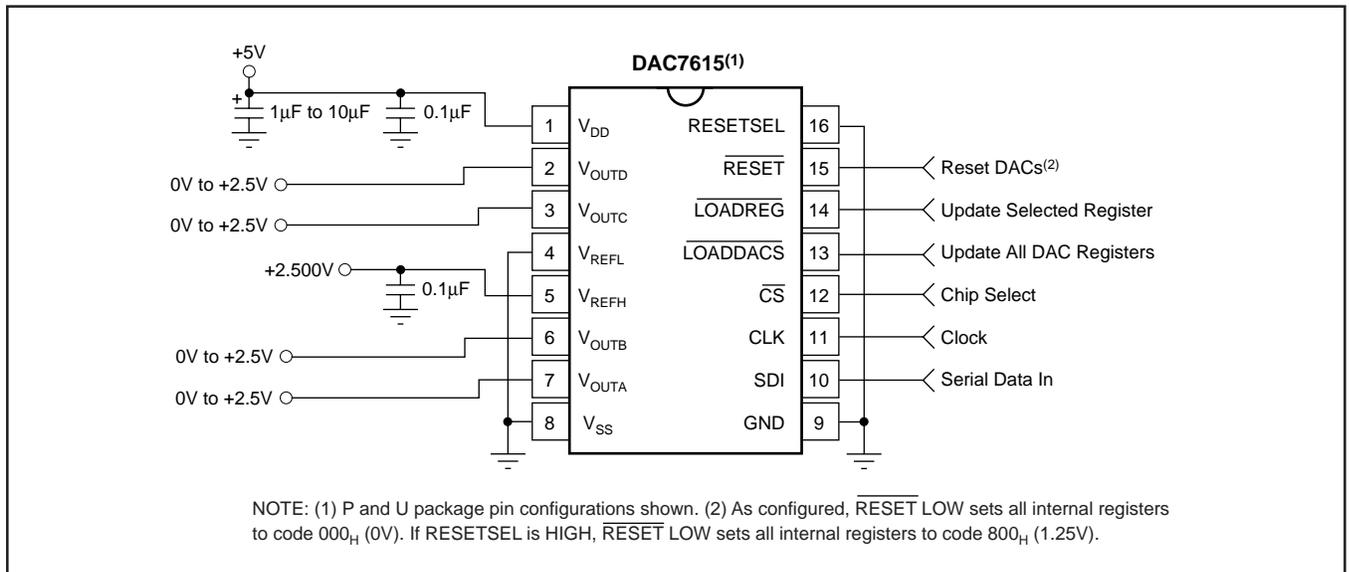
FIGURE 1. Basic Single-Supply Operation of the DAC7615.
