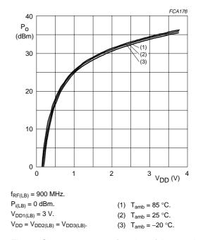
Fig.4 Output power as a function of the supply voltage.
