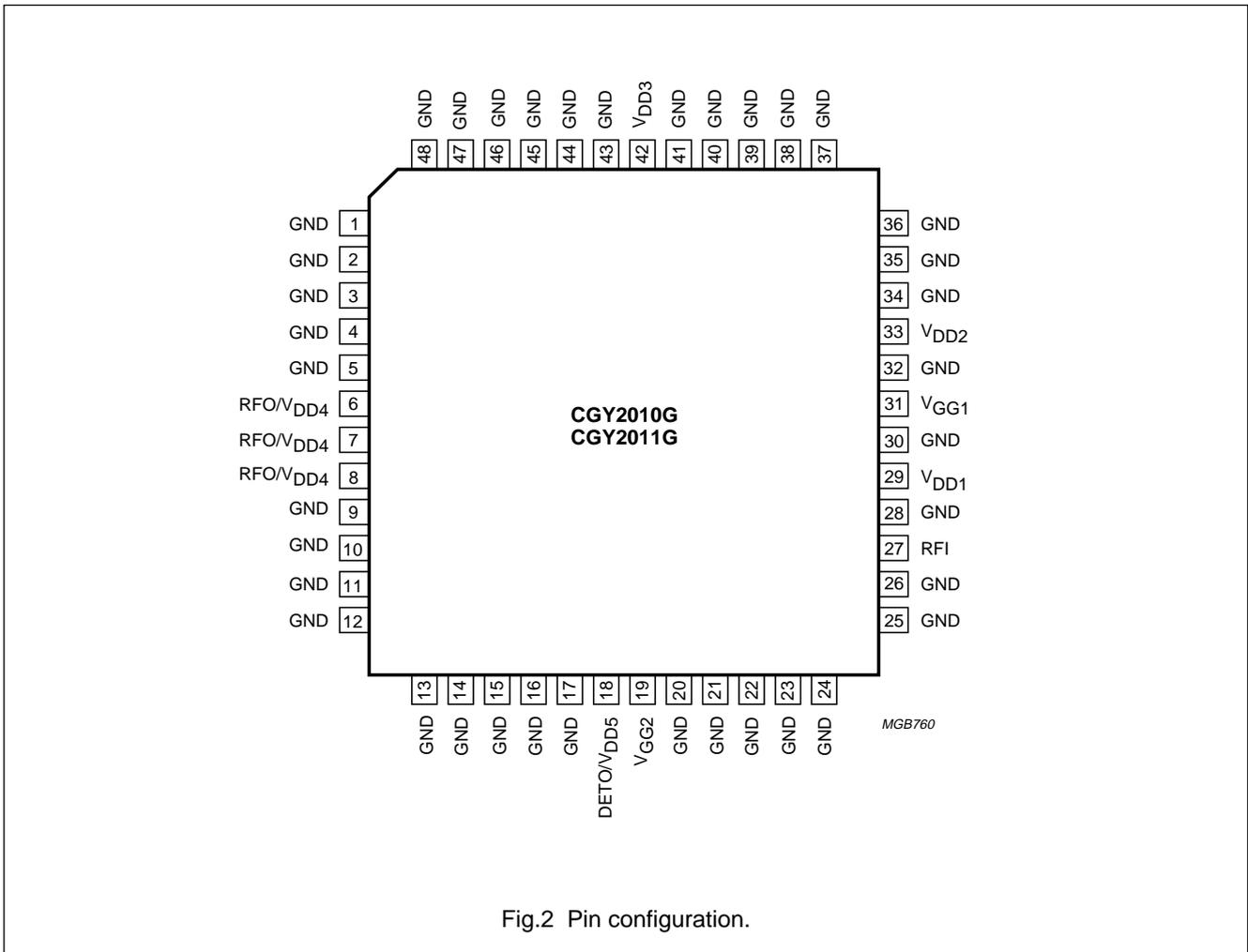
Fig.2 Pin configuration.
