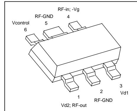
ESD: Electrostatic discharge sensitive device,
