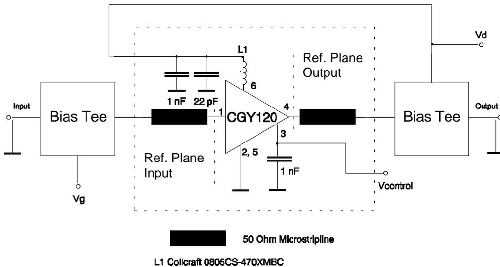
For optimized device performance, Vg has to be adapted ( $V_g \approx -1V \dots 0V$ ) to  $I \approx 45mA$  at Vd-supply under condition  $V_{control} = +2V$ .
