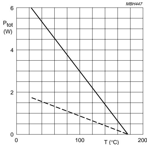
Solid line: tie-point temperature; lead length = 10 mm.
