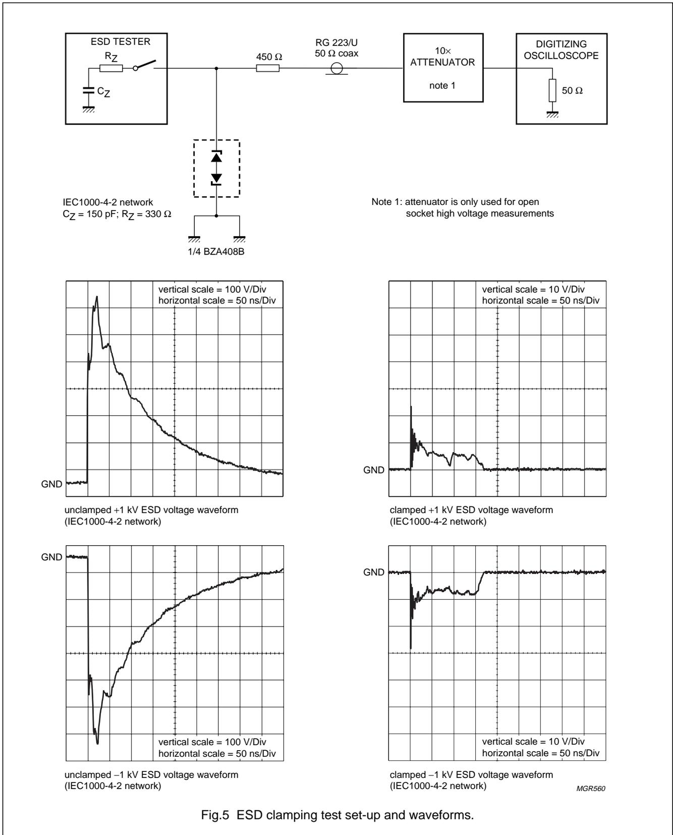
Fig.5 ESD clamping test set-up and waveforms.
