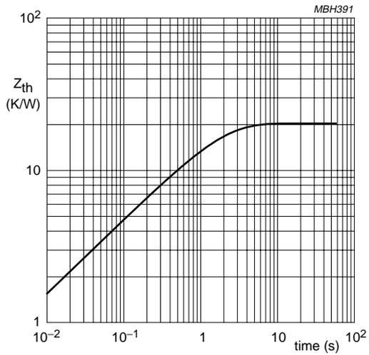
Fig.6 Thermal impedance in oil as a function of time.
