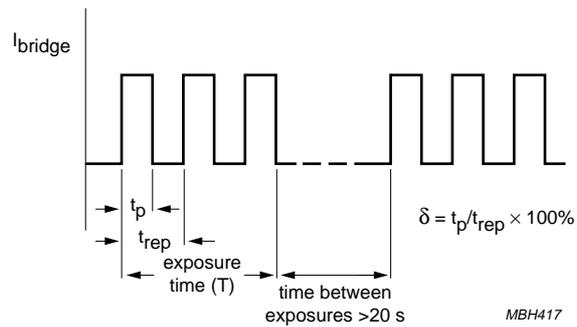
Fig.10 Maximum current through a 3-phase bridge rectifier versus pulse duration; exposure time  $T = 3$  s;
