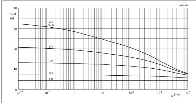
$T_{tp} = 50$ °C;  $R_{th j-tp} = 25$  K/W.
