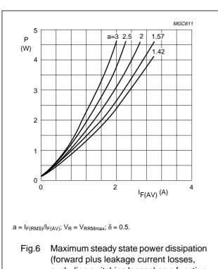
excluding switching losses) as a function of average forward current.
