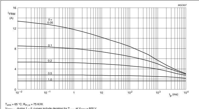
$V_{RRMmax}$  during 1 –  $\delta$ ; curves include derating for  $T_{j max}$  at  $V_{RRM}$  = 600 V.
