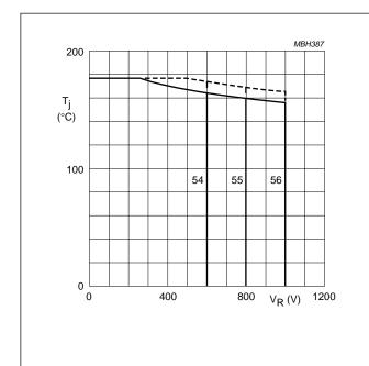
Solid line =  $V_R$ . Dotted line =  $V_{RRM}$ ;  $\delta$  = 0.5.
