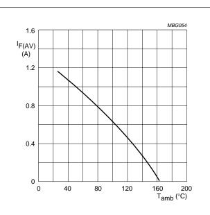
a = 1.57;  $V_R = V_{RRMmax}$ ;  $\delta$  = 0.5; device mounted as shown in Fig.9.
