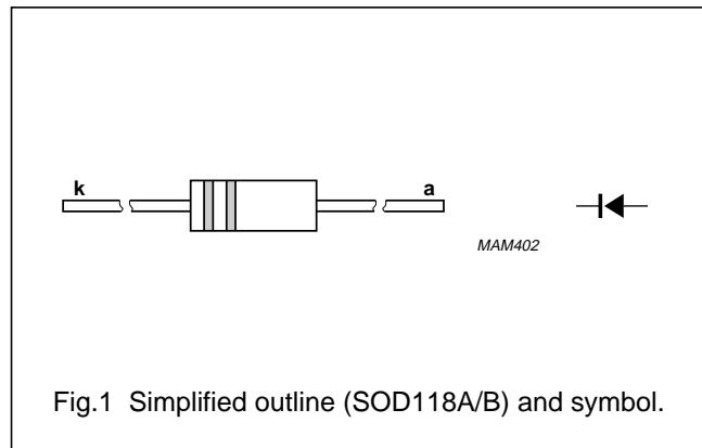
Fig.1 Simplified outline (SOD118A/B) and symbol.
