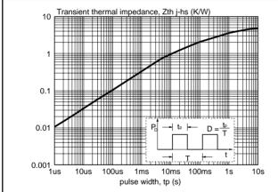
Fig.4. Transient thermal impedance  $Z_{th} = f(t_p)$
