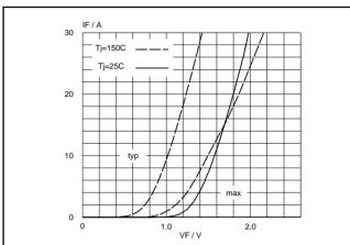
Fig.5. BY359F-1500 forward characteristic  $I_F = f(V_F)$ ; parameter  $T_j$
