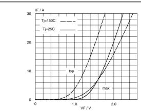
Fig.6. BY359F-1500S forward characteristic  $I_F = f(V_F)$ ; parameter  $T_i$
