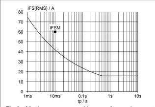
Fig.3. Maximum non-repetitive rms forward current.  $I_F = f(t_p)$ ; sinusoidal current waveform;  $T_j = 150^{\circ}C$  prior to surge with reapplied  $V_{RWM}$ .
