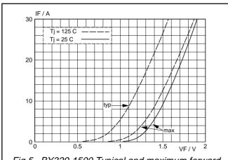
Fig.5. BY329-1500 Typical and maximum forward characteristic  $I_F = f(V_F)$ ; parameter  $T_j$
