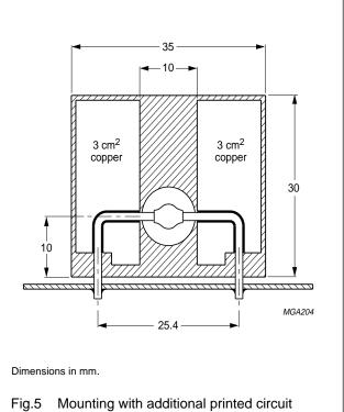
Fig.5 Mounting with additional printed circuit board for heat sink purposes.
