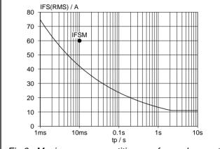
Fig.3. Maximum non-repetitive rms forward current.  $I_F = f(t_p)$ ; sinusoidal current waveform;  $T_j = 150^{\circ} C$  prior to surge with reapplied  $V_{RWM}$ .
