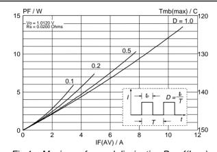
Fig.1. Maximum forward dissipation  $P_F = f(I_{F(AV)})$ ; square wave where  $I_{F(AV)} = I_{F(RMS)} \dot{x} \sqrt{D}$ .
