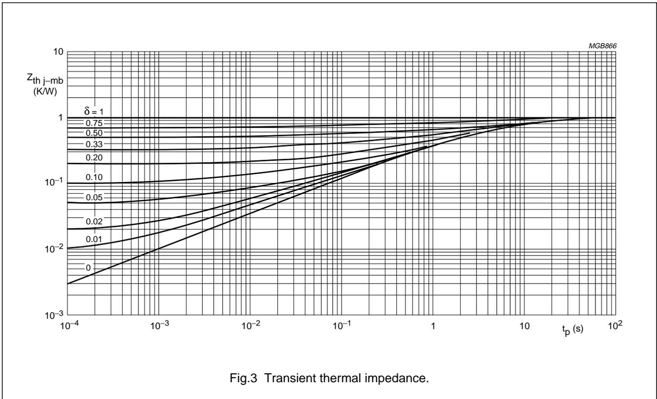
Fig.3 Transient thermal impedance.
