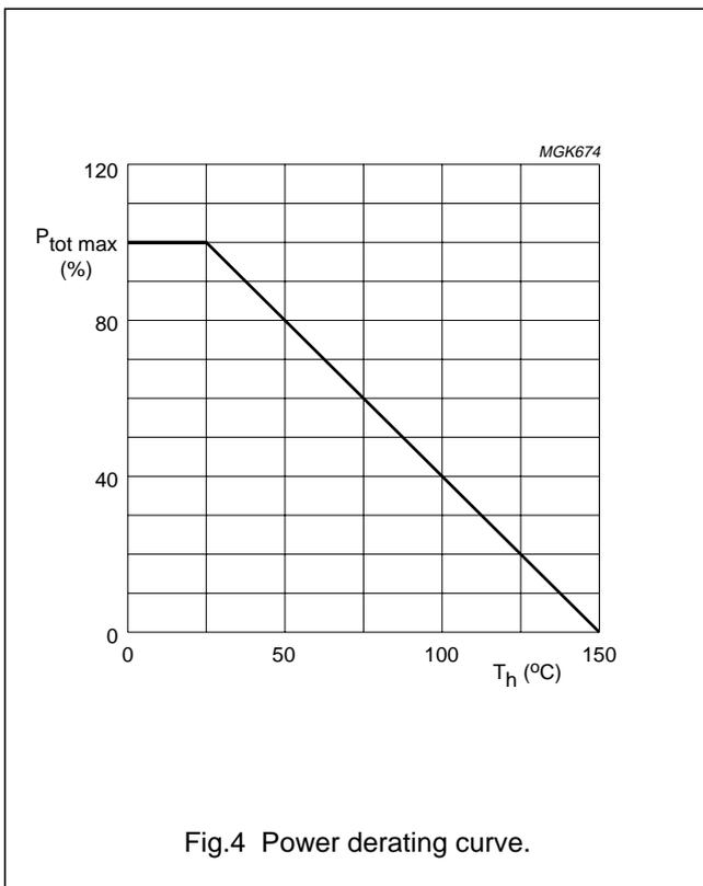
Fig.4 Power derating curve.
