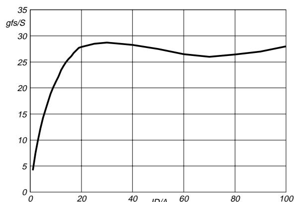
Fig.8. Typical transconductance,  $T_j = 25^\circ\text{C}$ .
