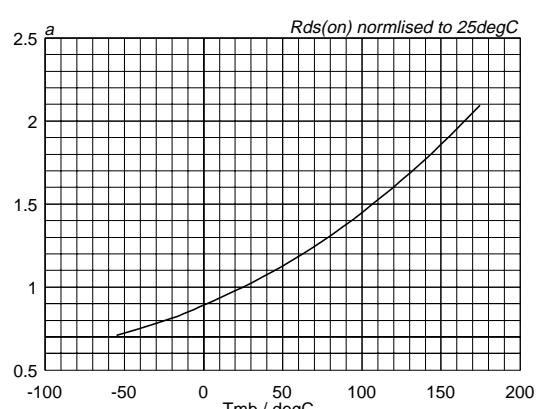
Fig.9. Normalised drain-source on-state resistance.
