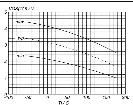
Fig.10. Gate threshold voltage.
