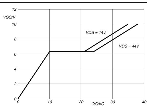
Fig.13. Typical turn-on gate-charge characteristics.
