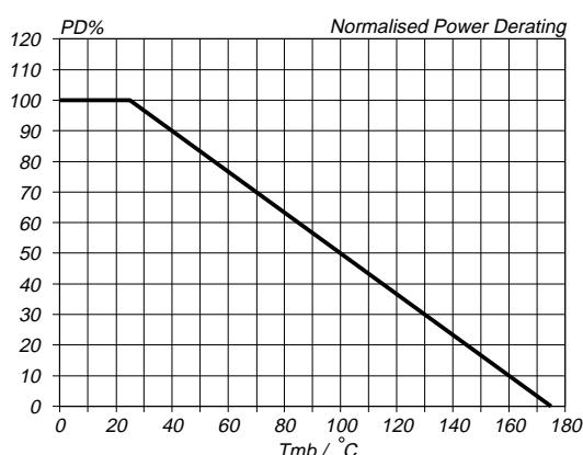
Fig.1. Normalised power dissipation.
