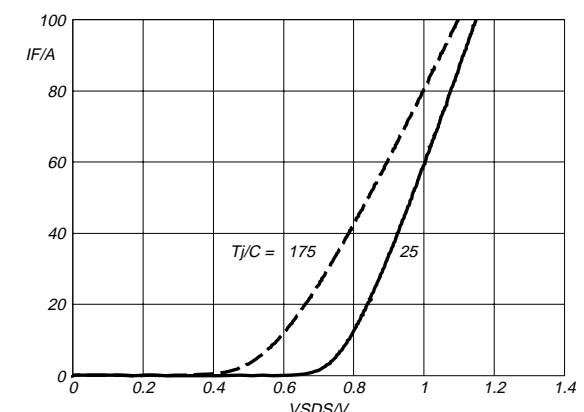
Fig.14. Typical reverse diode current.
