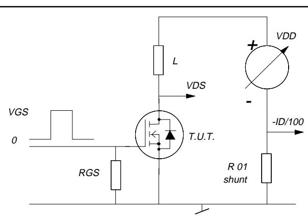
Fig.16. Avalanche energy test circuit.
