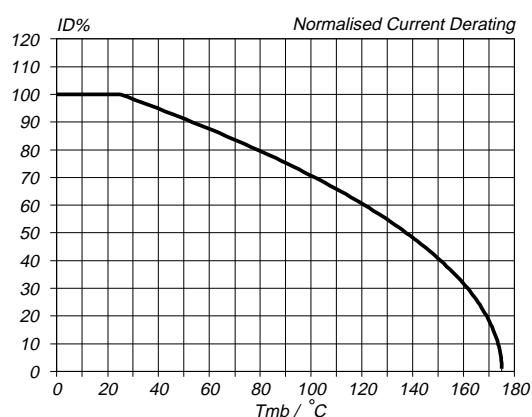
Fig.2. Normalised continuous drain current.
