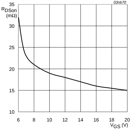
Fig 6. Drain-source on-state resistance as a function of gate-source voltage; typical values.
