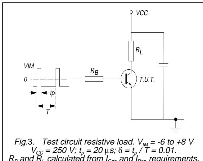
Fig.3. Test circuit resistive load.  $V_{IM} = -6$  to  $+8\text{ V}$
