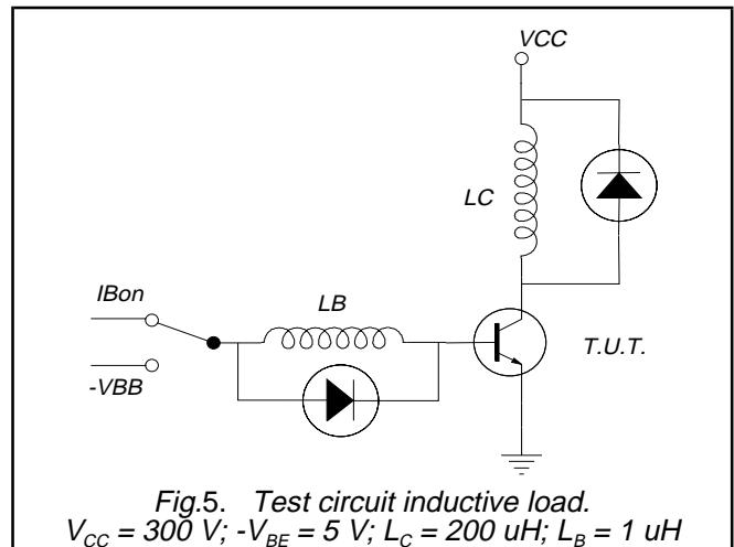
Fig.5. Test circuit inductive load.
