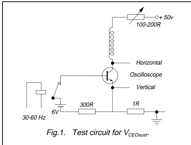
Fig.1. Test circuit for  $V_{CEO}$  sust.
