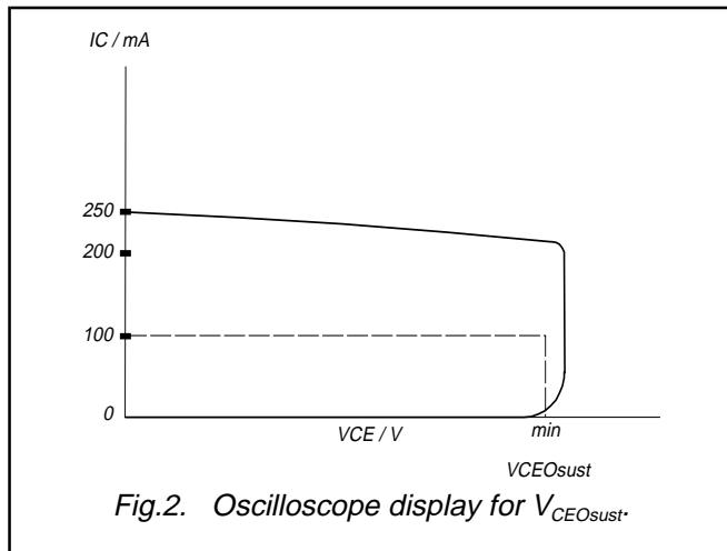
Fig.2. Oscilloscope display for  $V_{CEO}$  sust.
