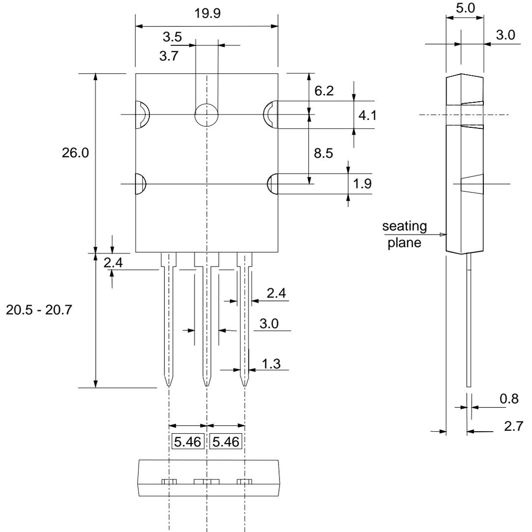
Fig.1. SOT430; pin 2 connected to mounting base.
