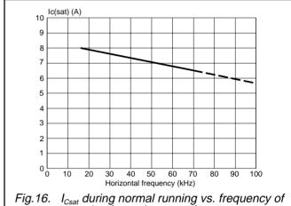
Fig.16. I<sub>Csat</sub> during normal running vs. frequency of operation for optimum performance
