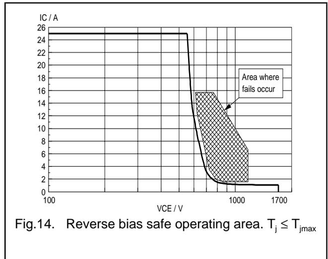
Silicon Diffused Power Transistor
