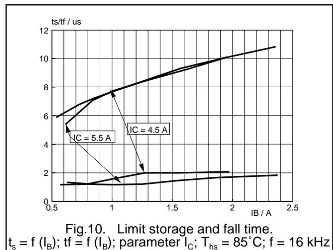
Silicon Diffused Power Transistor
