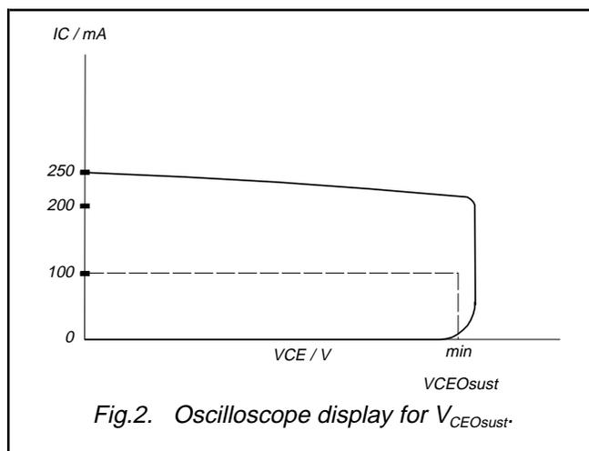
2 Measured with half sine-wave voltage (curve tracer).
