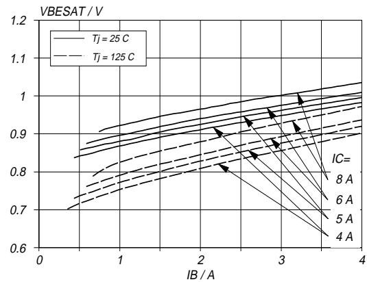
Fig.9. Typical base-emitter saturation voltage.
