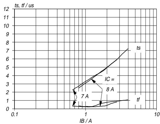
Fig.12. Typical collector storage and fall time.
