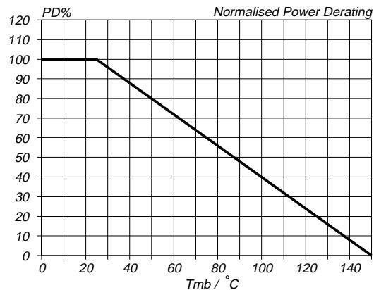
Fig.13. Normalised power dissipation.
