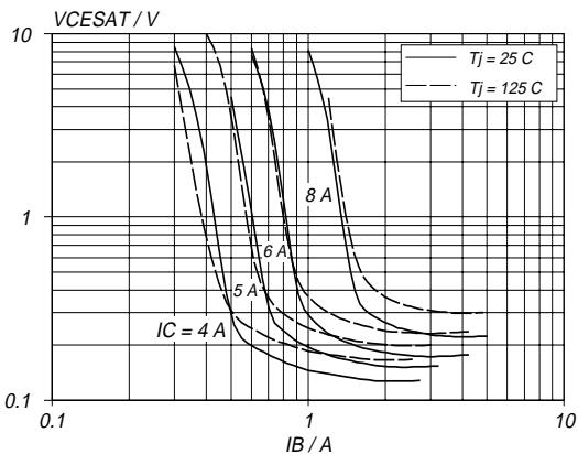
Fig.10. Typical collector-emitter saturation voltage.
