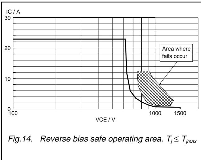
Silicon Diffused Power Transistor
