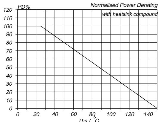
Fig.10. Normalised power dissipation.
