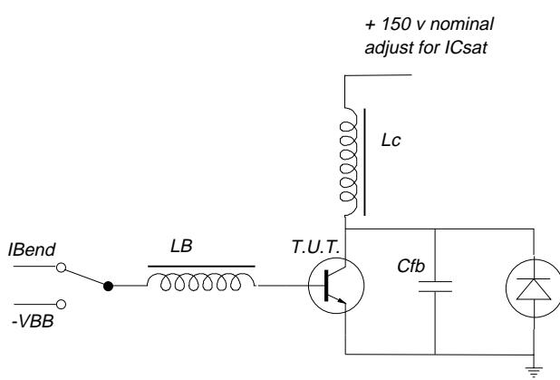
Fig.3. Switching times test circuit.
