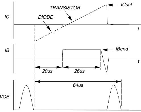
Fig.1. Switching times waveforms.
