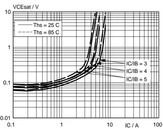
Fig.6. Typical collector-emitter saturation voltage.
