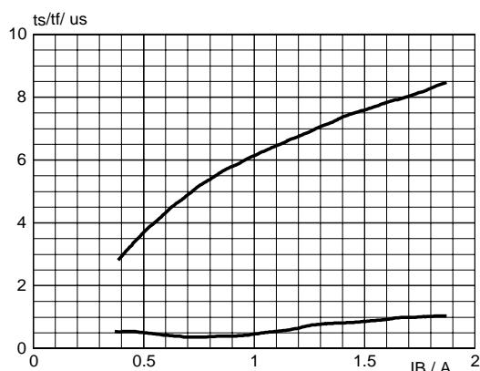
Fig.9. Typical collector storage and fall time.
