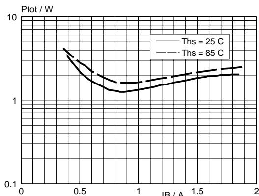
Fig.8. Typical losses.
