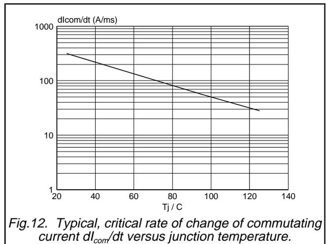
Fig. 12. Typical, critical rate of change of commutating current  $di_{com}/dt$  versus junction temperature.
