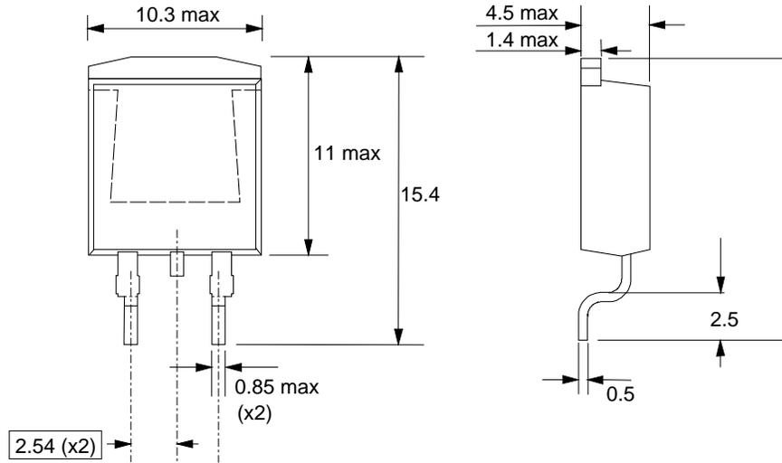
*Fig.13. SOT404 : centre pin connected to mounting base.*
