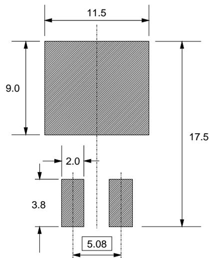
*Fig.2. SOT404 : minimum pad sizes for surface mounting.*
