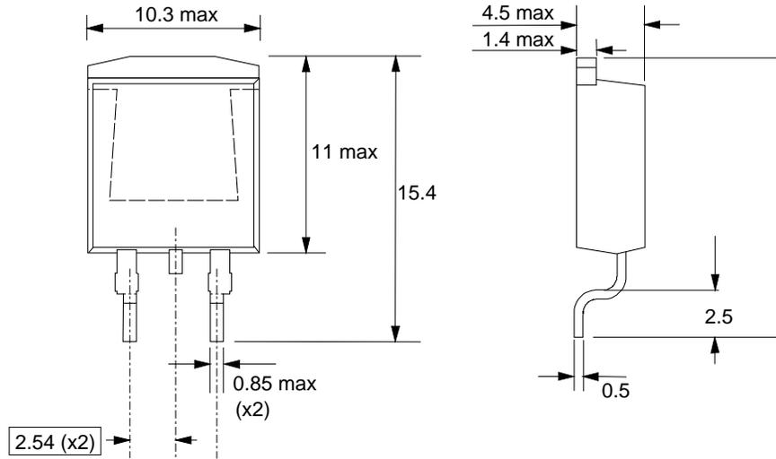
*Fig.1. SOT404 : centre pin connected to mounting base.*
