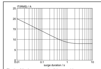
Fig.5. Maximum permissible repetitive rms on-state current  $I_{T(RMS)}$ , versus surge duration, for sinusoidal currents, f = 50 Hz;  $T_{hs} \le 73$ °C.
